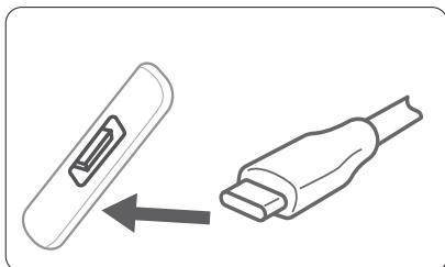
Insert the Type-C cable to initiate the charging process.
