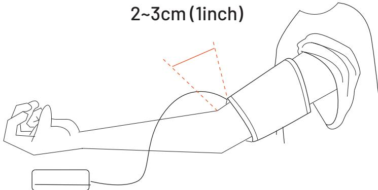
5. Align the air tube along the inner side of the arm, following the line of the middle finger.
